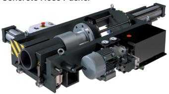
**Description:** Boasting 22,000 lbs of crimping force, the KPUSH22-CON is designed for difficult, heavy duty industrial hose such as concrete and petroleum hoses. Concrete hose mandrels and non-slip hose jaws sold separately.
