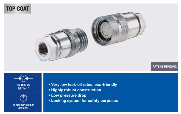
**General features:** ARGUS QS quick release couplings enable oil leak-free connection and disconnection of hydraulic lines. Their robust construction and tested components make them ideally suited for high and intermittent pressure loads. During the coupling action, valves that release and/or block the flow are automatically activated. The QS quick release coupling, formed by coupling plug and coupling socket, is coupled by a screwing action with the hand nut of the plug component.
