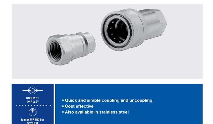
**General features:** ARGUS ISO 7241-1 series "A" quick release couplings are used for quick coupling and uncoupling of hydraulic lines. During the coupling action in zero or lowpressure ranges, valves that release or block the flow are automatically activated. The QA-ISO-A quick release coupling, formed by the coupling plug and the coupling socket, is connected by pushing on a sleeve. This guarantees a flush connection between the two coupling halves.
