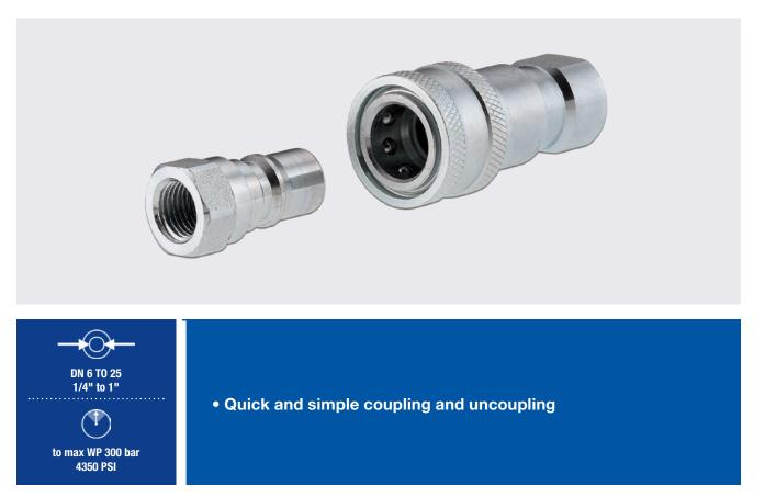
**General features:** ARGUS ISO 7241-1 series "B" quick release couplings are used for quick coupling and uncoupling of hydraulic lines. During the coupling action in zero or lowpressure ranges, valves that release or block the flow are automatically activated. The QB-ISO-B quick release coupling, formed by the coupling plug and the coupling socket, is connected by pushing on a sleeve. This guarantees a flush connection between the two coupling halves.
