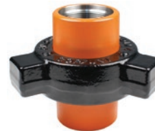
Figure 602 Threaded 6000 PSI CWP Specially Designed Lip Type Elastomer Seal Protects Metal to Metal Sealing Surface and Reduces Line Flow Turbulence
