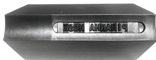
Marking Die Segment with Character Blocks inserted
