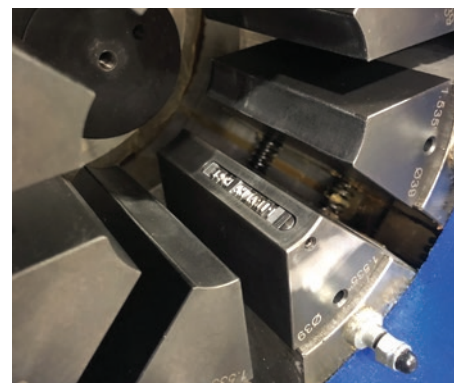
Marking Die Segments replace one of the eight standard die segments for that particular size (crimp diameter).
