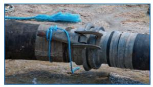
Non Sphere Lock handles tied down with rope, susceptible to unwanted opening.
