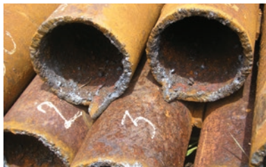
Well riser pipes showing signs of corrosion and scaling.
