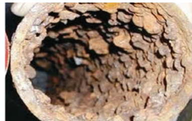
Well riser pipes showing signs of corrosion and scaling.
