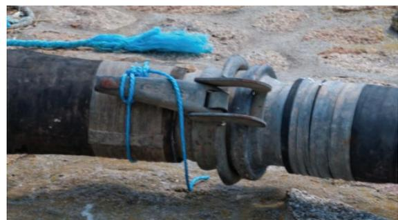
*Non Sphere Lock™ handles tied down with rope, susceptible to unwanted opening.*
